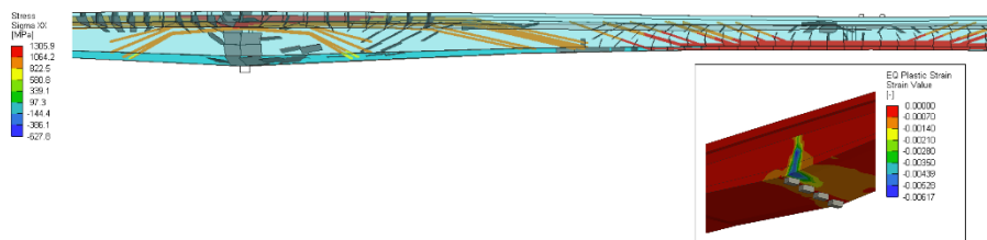
Fig. 3. Longitudinal view of the Wonka Bridge shows the stress in the bonded cables and cracks in the box girder at the peak load. The detail shows the development of the crushing zone above the support of the bridge.
